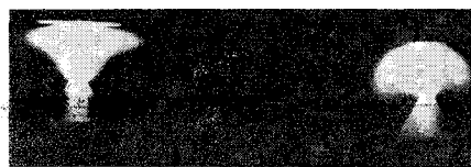
Fig. 2 Arc with transpiration-cooled anode. Left—Low-blowing Mode; right—Medium-blowing Mode.
